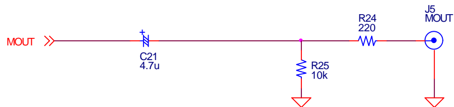
Figure 4. MOUT Output circuits
